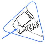
Toggle Mic ON - Press left side button after pairing (upwards audio cue is 'on' downwards audio cue is 'mute')
