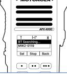
4. Press left side button (firmly) to put mobiWAN into Radio mode (hear audio cue: 'headset mode / radio mode')
